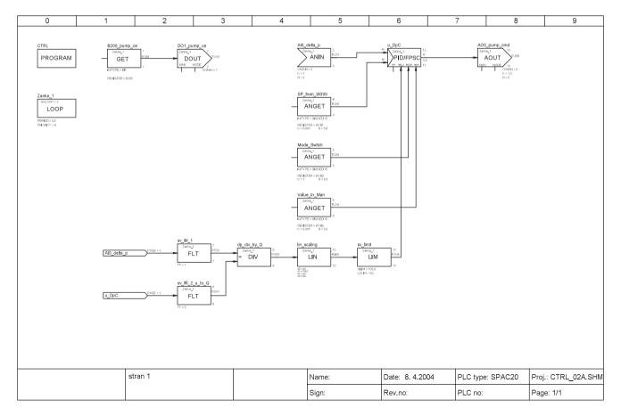
Fig. 9. Valve pressure control scheme designed using IDR BLOK.
