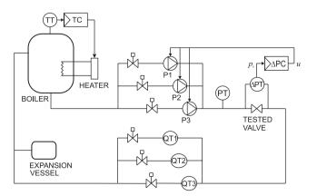
Fig. 6. Apparatus for testing of hydraulic valve (simplified).
